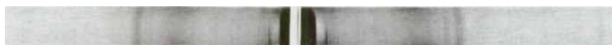
Figure 6. Powder pattern of compound 3d ( n = 12 ) recorded for the columnar, rectangular centred phase D_r upon heating just above the crystalline phase.
